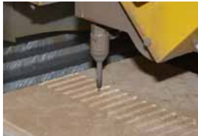
Bespoke slotted grilles being cut...
